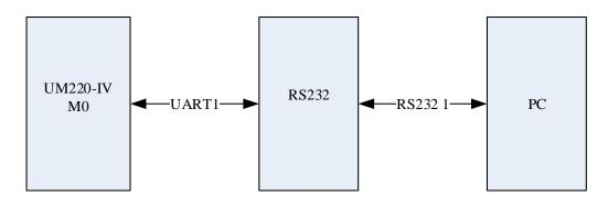
Figure 4-4 Connect COM to PC
