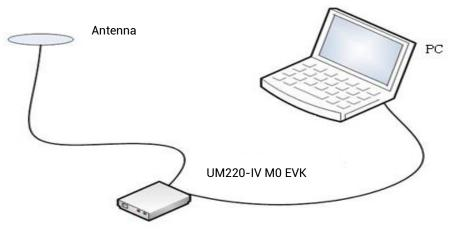
Figure 2-1 Typical Installation of UM220-IV M0 EVK
