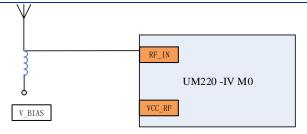
Figure 4-1 UM220-IV M0 Active Antenna Solution
