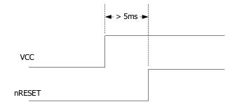
Figure 4-3 UM220-IV M0 Reset Requirement
